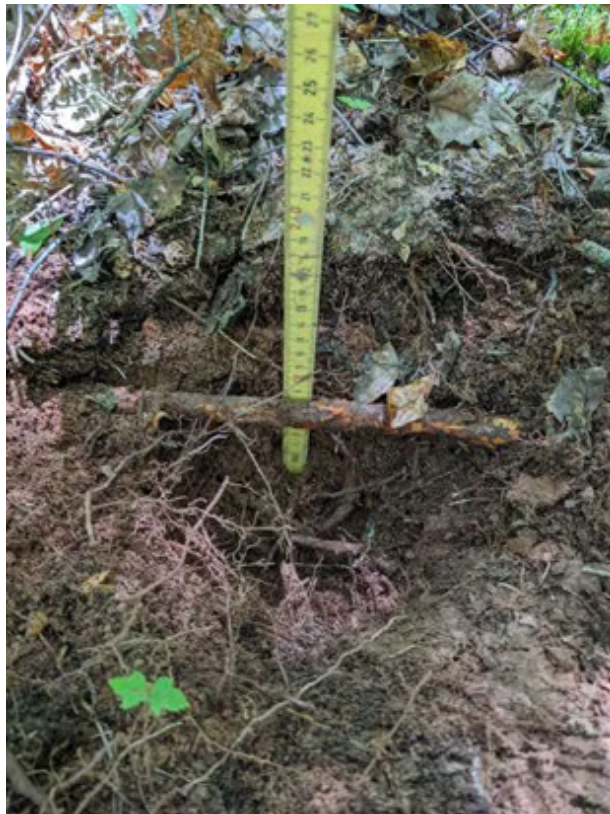
WL5 Photo 4 – Displaying upland soils (6-16 cm 2.5YR/4/6) with restrictive layer of roots at 16 cm
