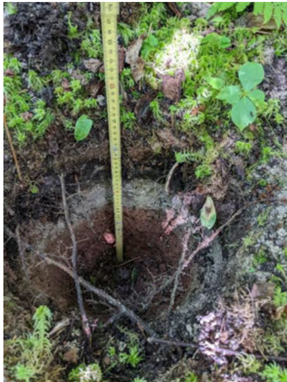
WL5 Photo 4 – Displaying Depleted Matrix (F3) soils (18-26 cm 5YR/8/1) with 3% redox features (5YR/6/8) over Red Parent Material (27-40 cm 2.5YR/4/3)
