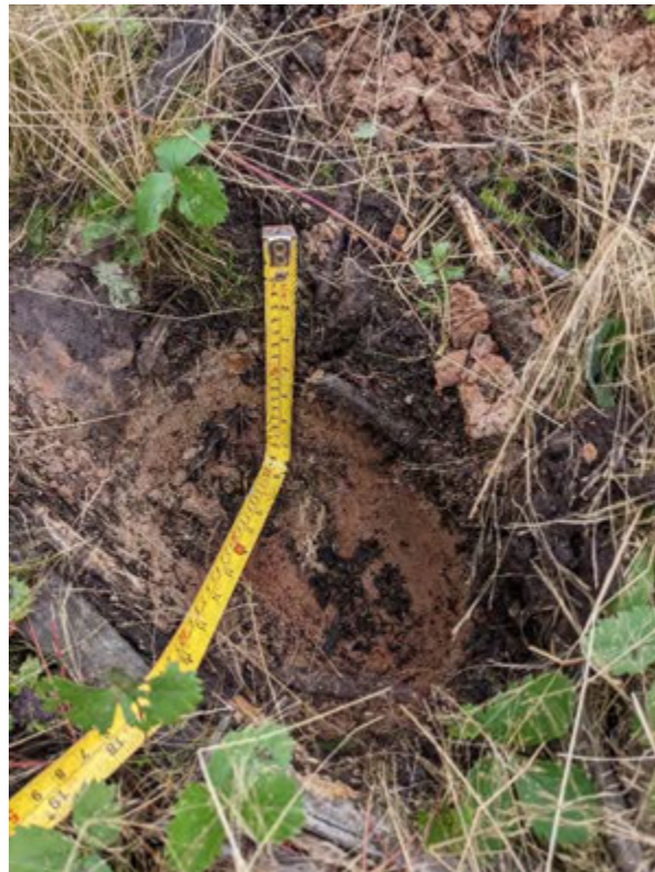
WL18 Photo 4 – Displaying Depleted Matrix (F3) (06-18cm 5YR/7/2) with 7% redox features (5YR/5/8) with a restrictive root layer at 18cm
