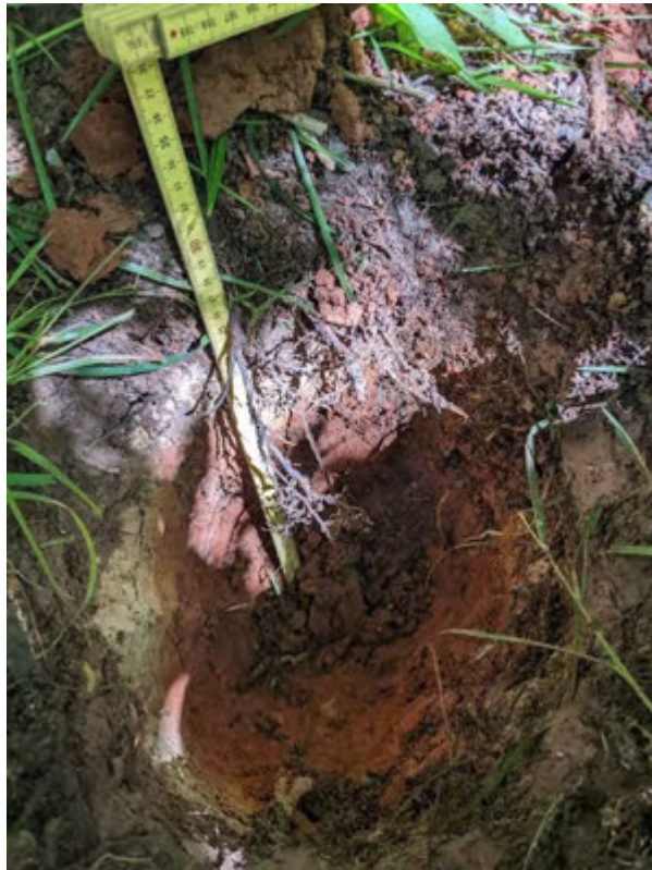
WL5 Photo 4 – Displaying Depleted Matrix (F3) soils (10-17 cm 2.5YR/6/1) with 20% redox features (5YR/6/8) over Red Parent Material (18-33 cm 2.5YR/4/3) with 2% redox features (2.5YR/6/8)
