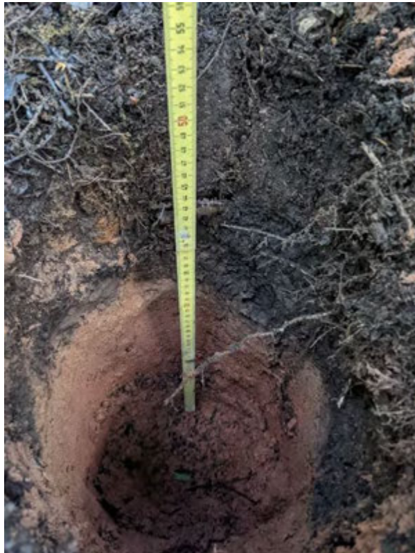
WL4 Photo 4 – Displaying Histic Epipedon (A2) soils (21-22 cm 5YR/4/2) with 2% redox features (5YR/6/8) over Red Parent Material (23-55 cm 7.5YR/4/4)
