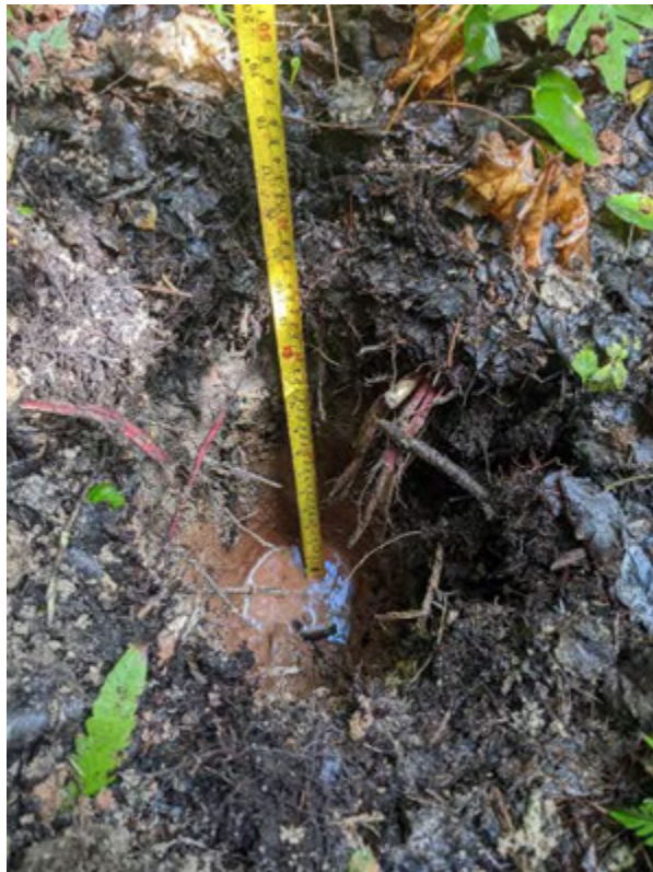
WL15 Photo 4 – Displaying Depleted Matrix (F3) (10-20cm 5YR/6/1) with 5% redox features (5YR/6/8) over Red Parent Material (21-40cm 2.5YR/5/4)
