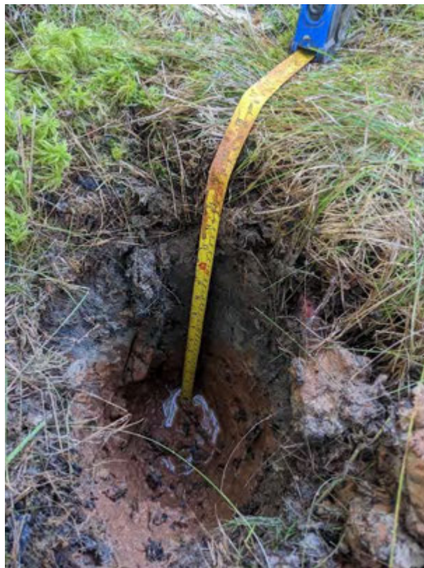
WL11 Photo 4 – Displaying Red Parent Material (2.5YR/3/5) with 7% reduct features (2.5YR/4/8) with water table at 40cm
