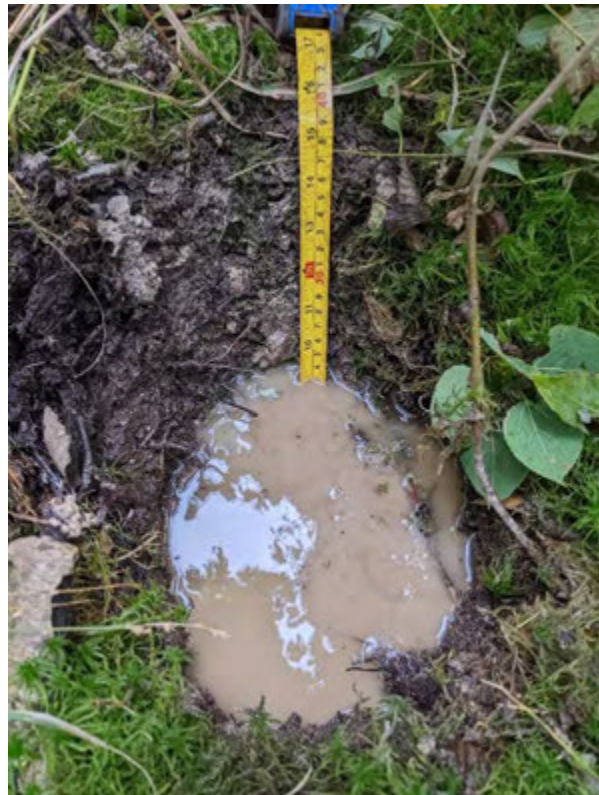
WL19 Photo 4 – Displaying Depleted Matrix (F3) (13-35cm 5YR/5/6) with 10% redox features (5YR/5/6) with water table at 12cm
