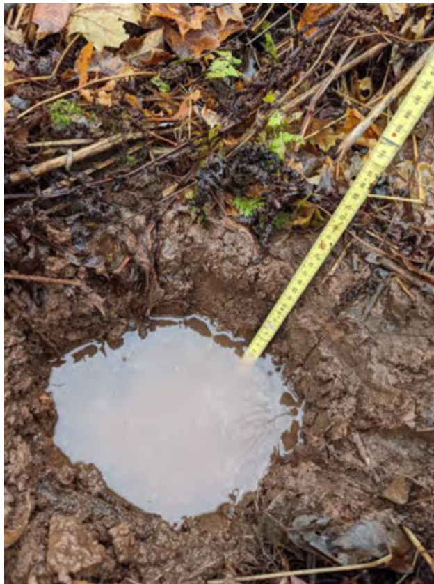
WL22 Photo 4 – Displaying Red Parent Material (F21) soils (03-25cm 5YR/3/3 with 5% undetermined redox features with water table at 15 cm
