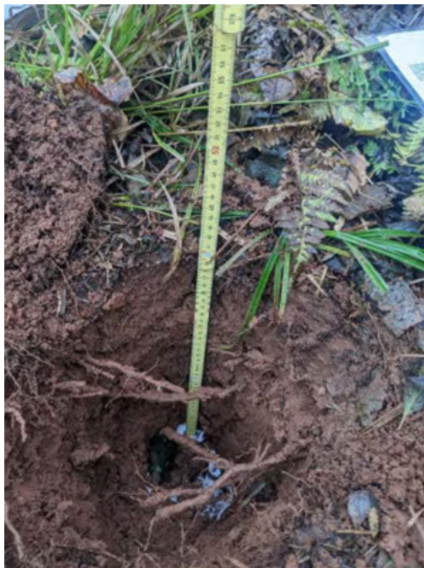
WL20 Photo 4 – Displaying Red Parent Material (F21) soils (2.5YR/4/4) with 5% undetermined redox features and water table at 40cm for WL20
