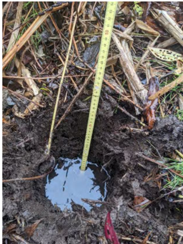
WL21 Photo 4 – Displaying Histosol (A1) soils (0-40cm 7.5YR/2.5/1) with water table at 30cm
