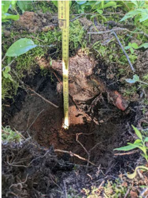
WL1 Photo 5 – Displaying Depleted Matrix (F3) soils (13-28cm 10YR4/2) with 10% redox features(5YR4/6) over Red Parent Material (29-37cm 5YR4/6)
