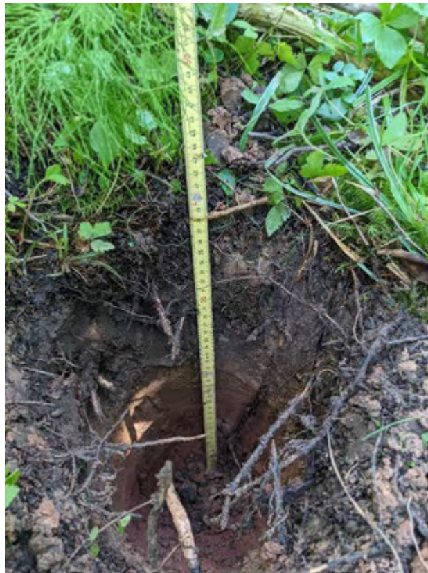
WL8 Photo 4 – Displaying Depleted Matrix (F3) soils (14-19cm 5YR/3/1) with 7% redox features (5YR/7/8) over 20-30 cm 5YR/4/4 with 2% redox features (7.5YR/6/6) over Red Parent Material (31-43cm 2.5YR/4/4)
